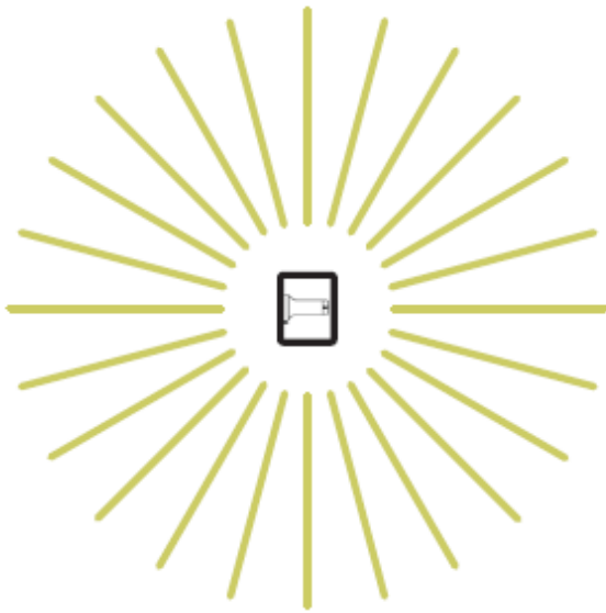
FIGURE 5 Typical AP Omni Coverage, Top View - Azimuth Plane Coverage
