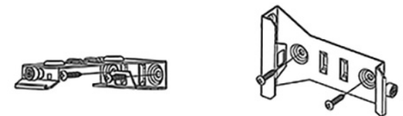
FIGURE 9 Mounting Bracket on a Flat Surface
